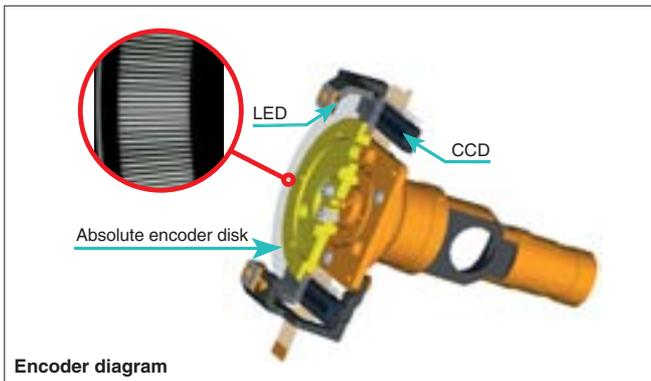
The Series30R models are equipped with Sokkia-developed absolute encoders. These encoders feature the RAB (RANdom Bi-directional) code technology first used in the SDL30 digital level, which provides high stability and reliability. You do not need to reset for 0 indexing at the start of a job, so surveying can begin from the moment you turn on the power. Work efficiency is also boosted by the immediate display of azimuth whenever you restart the total station.
