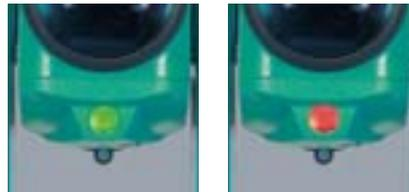
The Guide Light Unit GDL1 boosts efficiency of setting-out measurements. Its guide light is composed of two lights of different colors that are emitted from one aperture. When you are on the left side, the green light is visible, and when you are on the right side, the red light can be seen. When green and red are flashing back and forth, you are on the telescope sighting direction.
