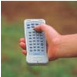
Protection against dust and water is another advantage, as you can use the keyboard without worry in the rain or at a dusty construction site. (IP44 compliant)
