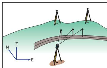
The Series30R performs three-dimensional setting out with N, E and Z or E, N and Z coordinates. Directions and distances to the setting out position are indicated on the screen.
