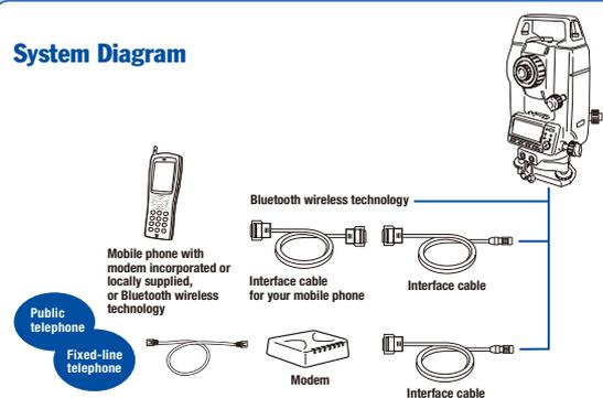
SFX requires connectivity using a mobile phone with a service provider capable of e-mail data transfer to an external source, as well as an active e-mail account and/or FTP server. Consult your local telecoms operator for proper equipment and connectivity requirements.
