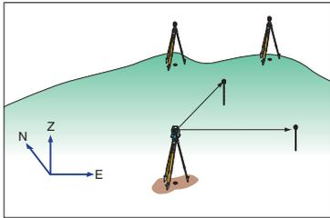
The Series30R calculates 3-D coordinate values of measuring points and displays them either as N, E, Z or E, N, Z.
