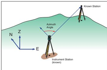
The Series30R can automatically set the horizontal angle to the azimuth of a back sight by using the coordinates of the instrument station and the back sight point.
