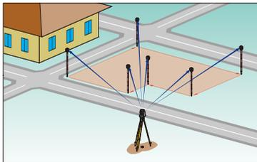
The Series30R can use measured points or stored data—up to 50 points in total—to calculate an area. Area calculations are made with 3D coordinates, so even sloped surfaces can be measured with ease and precision.
