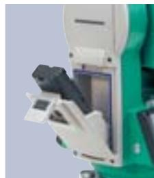
Take 7 hours of continuous angle and distance measurements with the Series30R's rechargeable lithium-ion battery. Unlike Ni-Cd cells, the Series30R's battery can be fully recharged at any time, without diminishing its energy capacity. The BDC46A battery is commonly used for Sokkia's Series10 total stations, digital levels, and other equipment.
