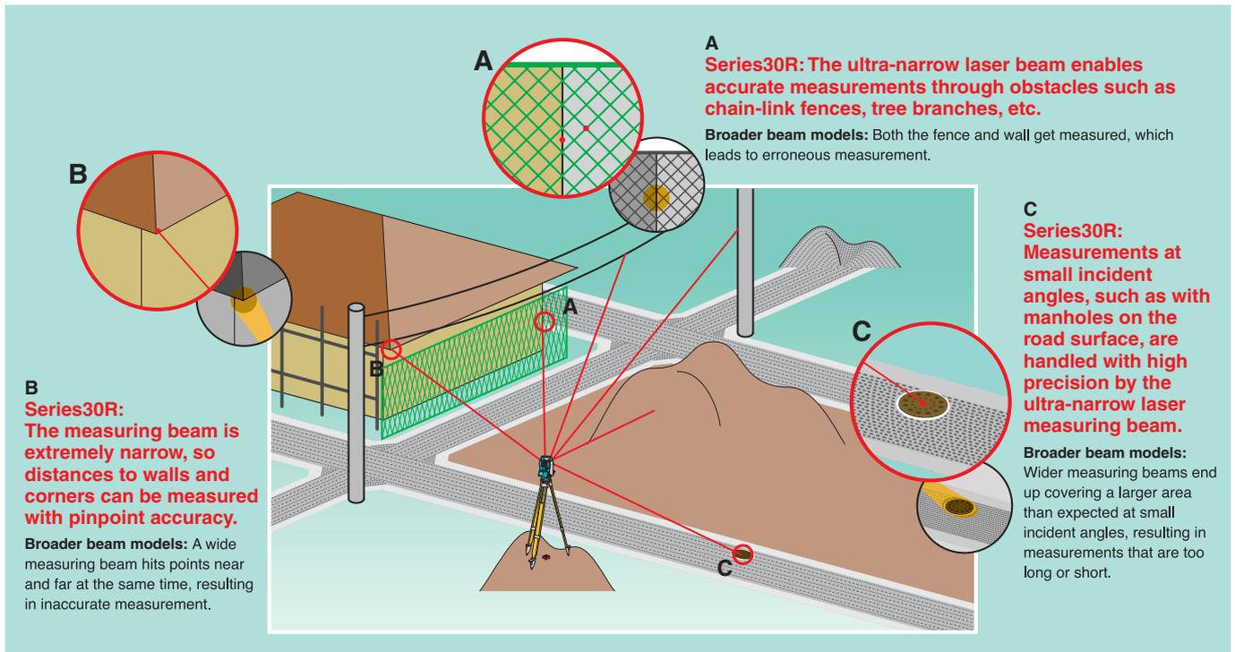
The Series30R employs an ultra small-diameter visible laser to obtain measurements with pinpoint accuracy. Fine objects, as well as the corners of walls and other structures, can be measured precisely. You can also make accurate measurements through obstacles such as chain-link fences and tree branches.
