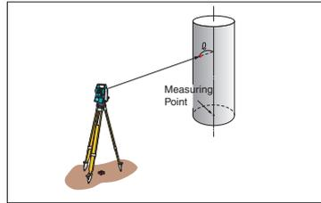
The Series30R calculates the angles and distance, or the coordinates of the measuring point by inputting the distance and direction between the measuring point and the offset point.
